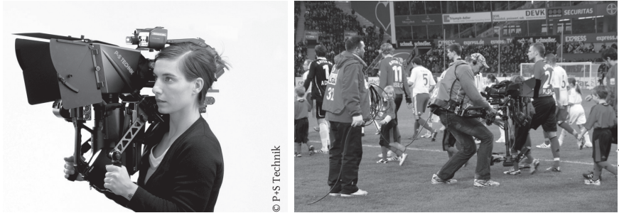
Setup with camera under: on the left, shoulder-mounted rig; on the right, Steadicam mounted rig.
